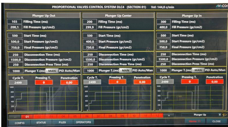
It can control up to 12 valves per section. Built with open standards and respecting the strictest CE safety and quality standards. Protected outputs against short circuit with automatic reset and opto coupled. Authorization level and management and maintenance programs. Continuous measurement of the position accuracy of the motors. High repeatability of production. According to European Regulation.
